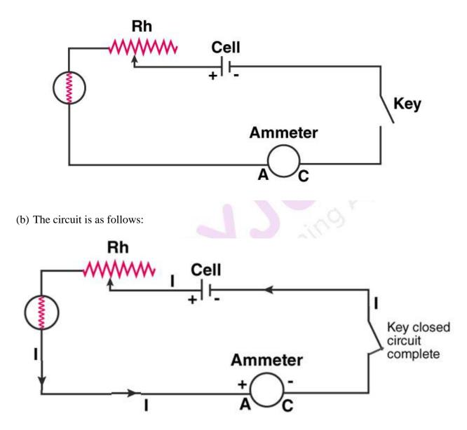
(c) Rh is the rheostat. Rheostat controls the flow of current in a circuit.
